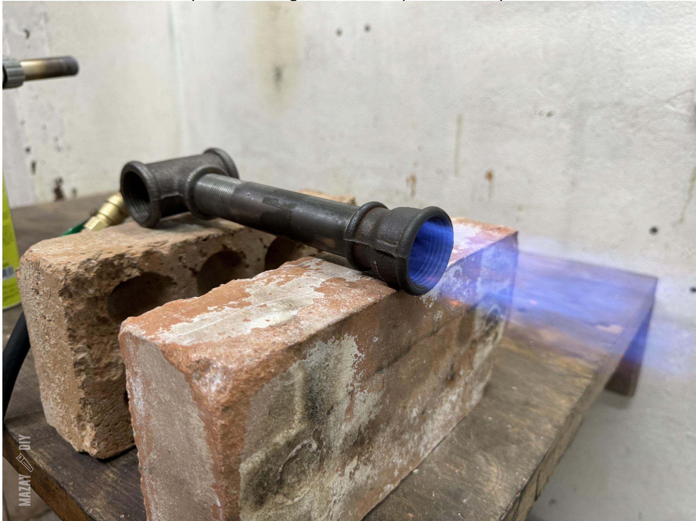
This simple T Burner originally designed by Frosty
